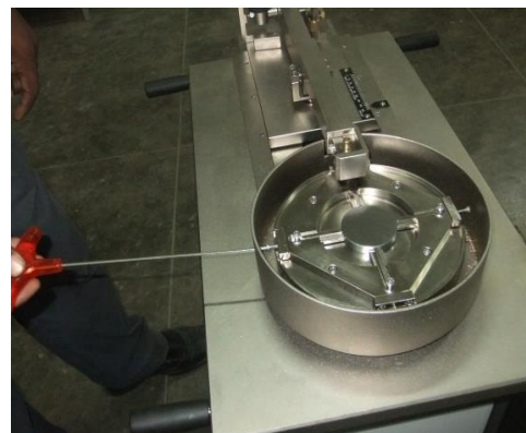
Fig. 1 Pin on disc wear test setup
