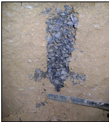
Mode of failure for L/D ratio of 4.
