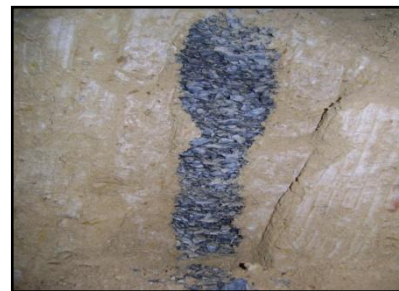
Mode of failure For L/D ratio of 6.1
