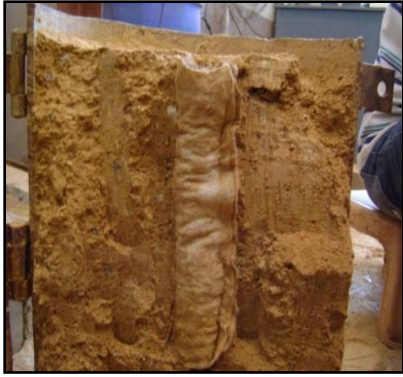
Reinforced stone column after test L/D=6.1
