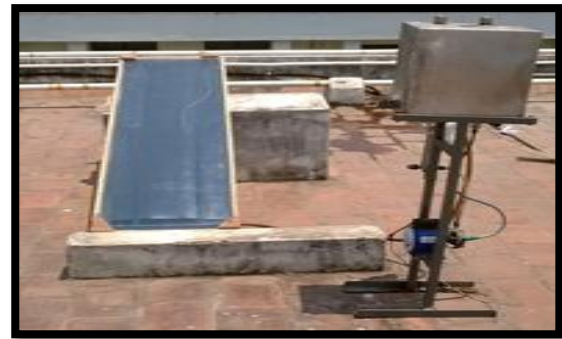
Fig. 1. Experimental setup of FPC with inner grooved and plain tube
