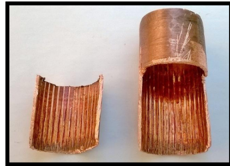
Fig.4. Inner view of grooved pipe
