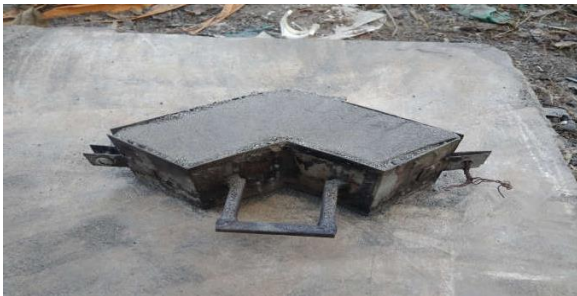
Fig.4 Casting of Paver Block
