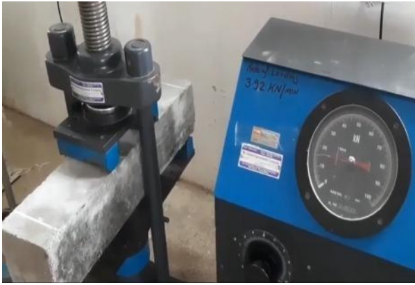
Fig. 6. Flexural-strength test setup photograph supplied in the report.
