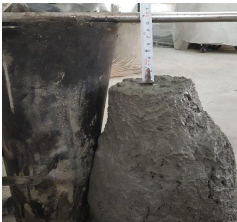
Fig. 2. Fresh concrete/slump observation photograph from the supplied report.
