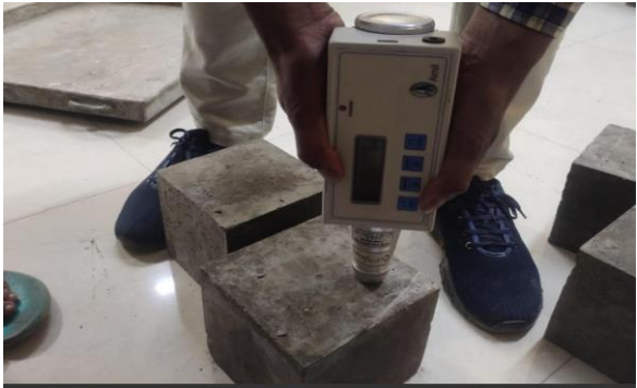
Fig. 9. Rebound hammer testing photograph supplied in the report.
