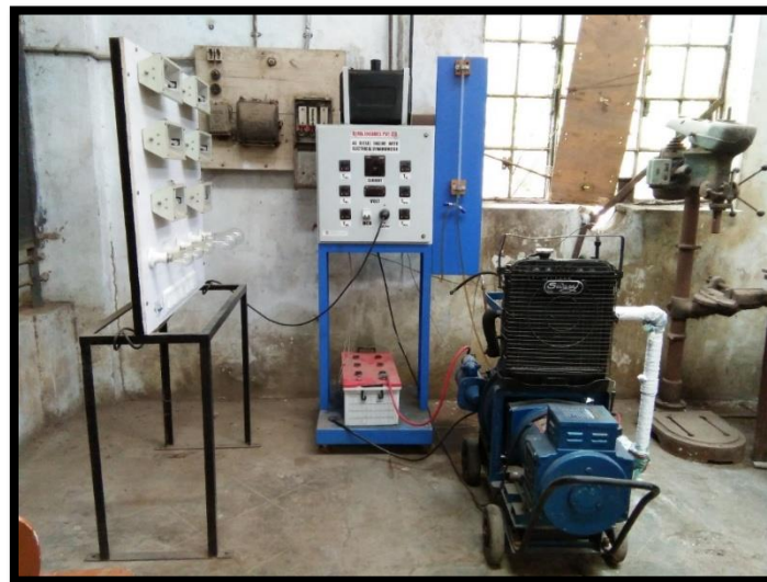
Figure 2. Photographic view of the experimental engine test rig illustrating the arrangement of dynamometer, fuel measurement system, and temperature sensing devices.
