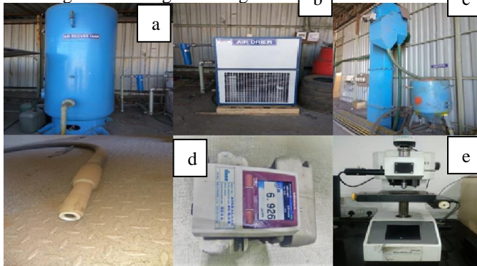
Figure 2. a) Air receiver tank, b) Air Drier, c) Hoper Unit, d) Surface roughness testing and e) Clemex Microhardness tester.
