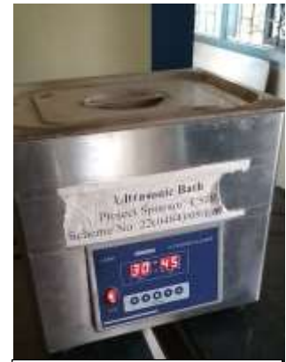
FIG 1c: nHTF IN ULTRASONIC BATH
