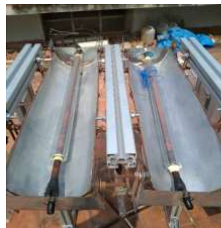
FIG 1g: FLUIDS IN COPPER TUBE ENCLOSED IN EVACUATED TUBE
