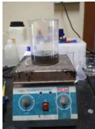
FIG 1b: DISPERSION OF CNT USING MAGNETIC STIRRER
