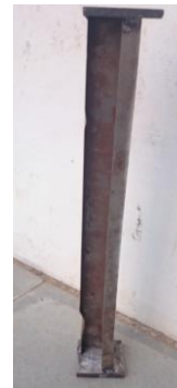
Figure7 Specimen After buckling
