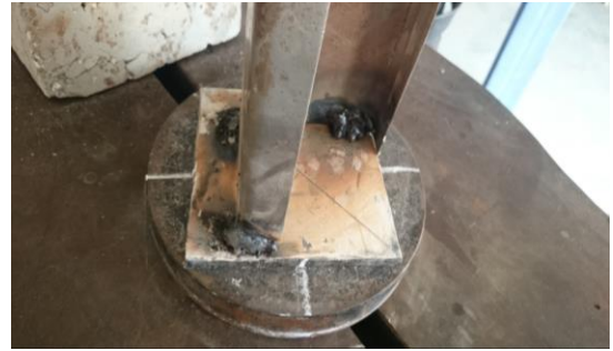
Figure 4 Marking of centroid of specimen & loading plate
