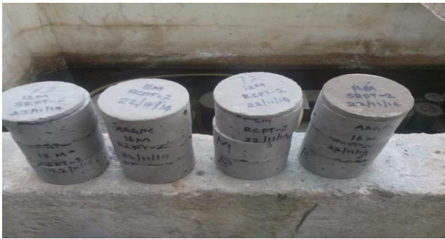
Fig:4.19: Specimen Left To Dry After Cutting
