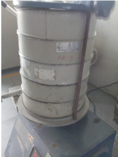
Fig:3.4: Coarse Aggregate Sieve Setup
