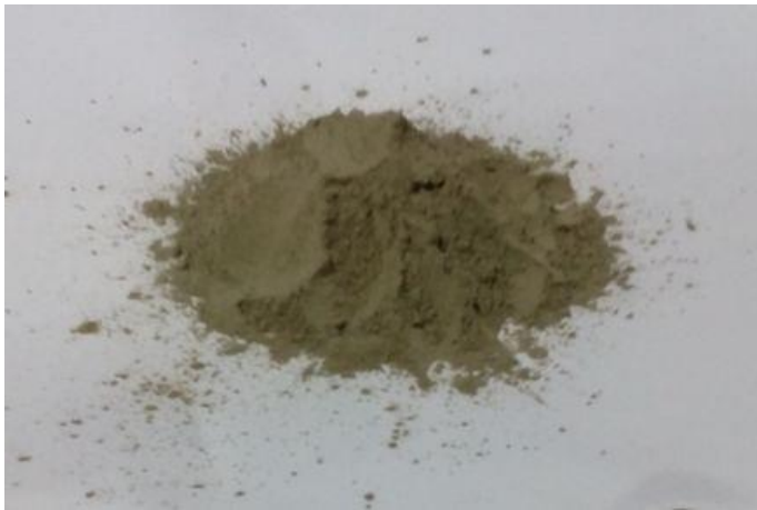
Fig:3.3: Ordinary Portland Cement(OPC 53Grade)
