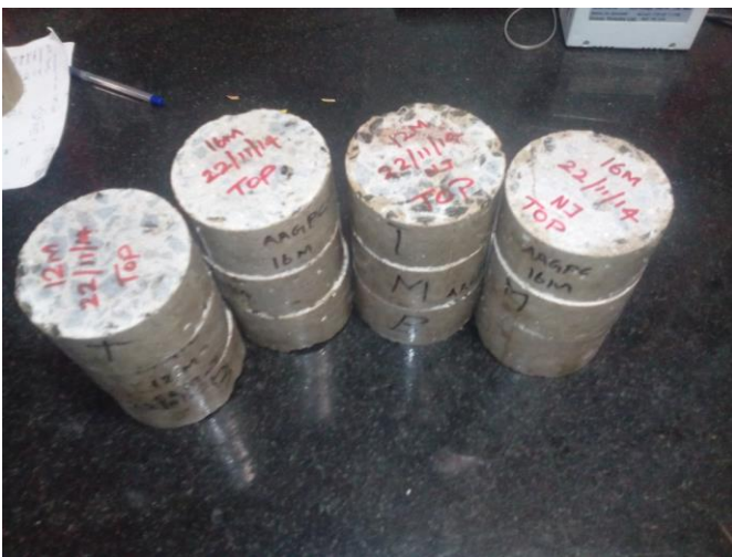
Fig:4.20: Specimens Painted With Epoxy
