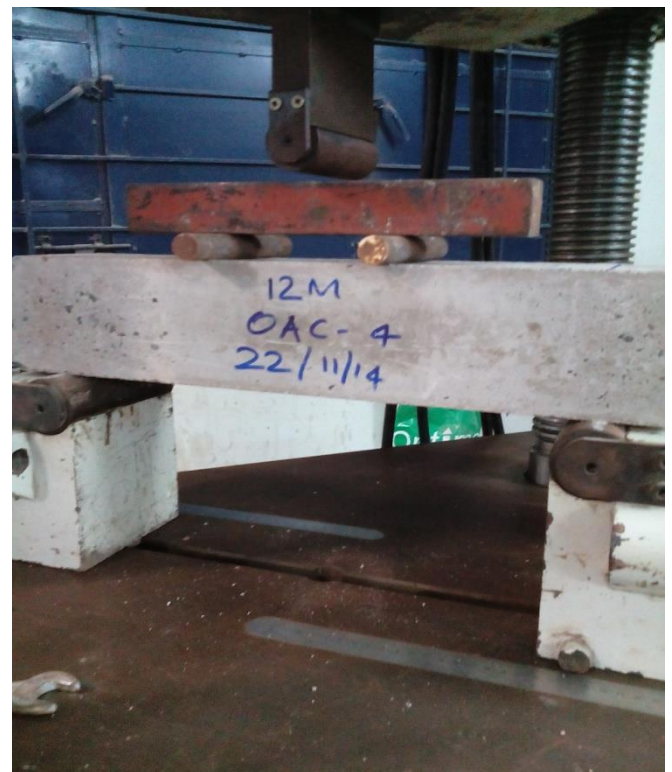
Fig:4.14: Flexural Testing Of Specimen
