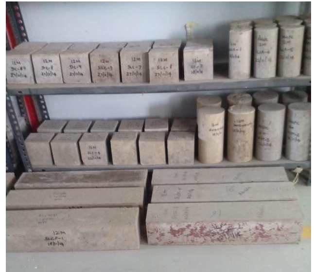
Fig:3.21: Specimens Left At Ambient Temperature (Open Air Curing)
