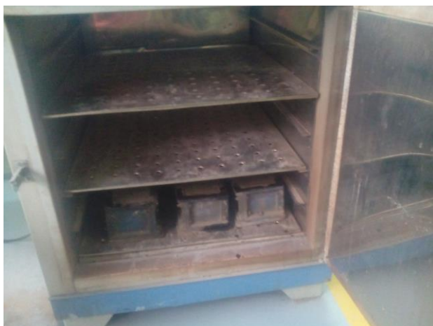
Fig:3.20: Specimens Cured In Hot Air Oven (Dry Curing)
