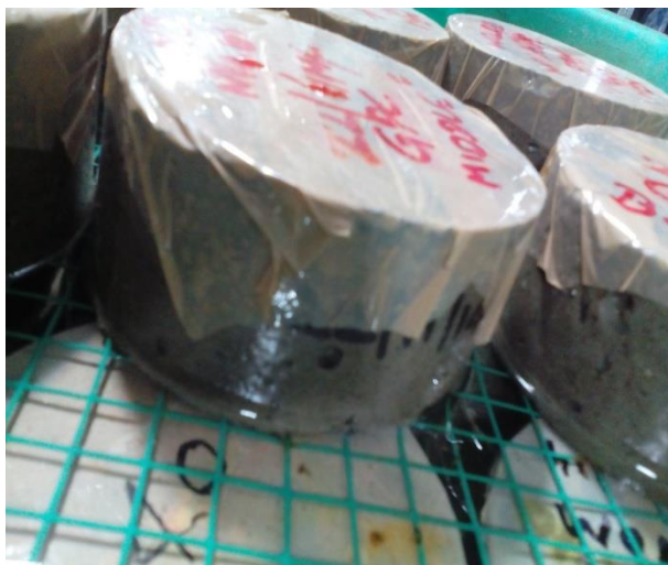
Fig:4.24 Specimens Been Epoxy Coated And Tapped At Top Surface
