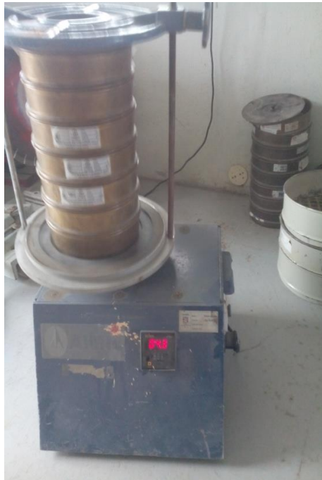
Fig:3.5: Fine Aggregate Sieve Setup
