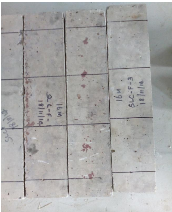
Fig:4.12: Marked Specimens For Flexural Test
