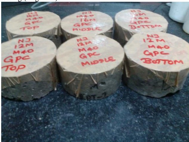
Fig:4.24 Specimens Been Epoxy Coated And Tapped At Top Surface
