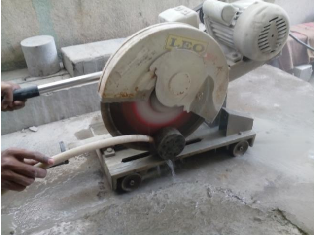
Fig:4.18: Specimen Cut Using Wet Cutting Blade
