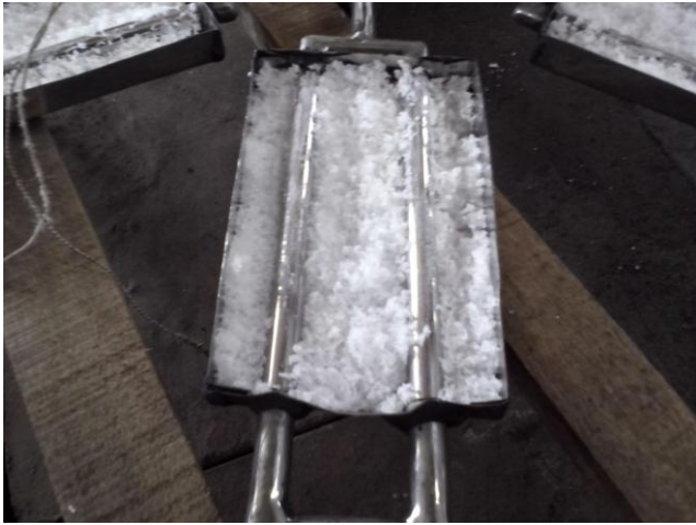
Fig 2. Tray half filled with MgCl_2 \cdot 6H_2O , double pipe passing through tray visible
