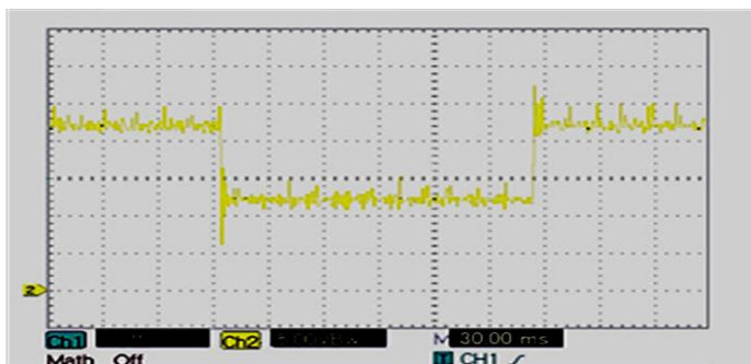
Figure 11 Experimental voltage responses with FO-PI controller for variable reference command
