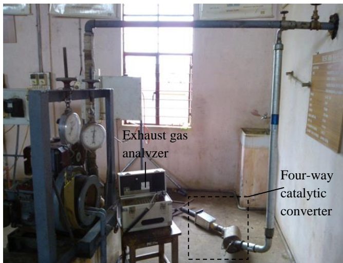
Fig.5. Diesel engine with four-way catalytic converter for experimental set up
