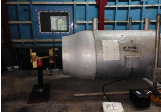
Fig.1 Open blower and mini VAWT for testing
