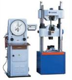
THREE POINT LOADING: The example is set on the roller gave in the bed of the UTM demonstrate that the example is precisely on the focal point of the roller. At that point step by step expanding load is connected until the point that the example falls flat. As the heaps connected the comparing diversion are taken from the dial gage settled to the UTM.
