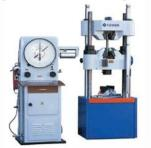
Three Point Loading: The example is set on the roller gave in the bed of the UTM demonstrate that the example is precisely on the focal point of the roller. At that point step by step expanding load is connected until the point that the example falls flat. As the heaps connected the comparing diversion are taken from the dial gage settled to the UTM.
