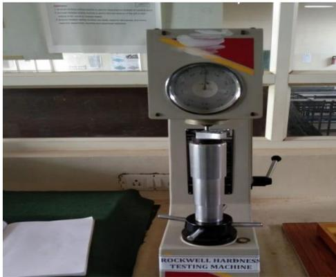
Fig 10 Rockwell Hardness Machine
