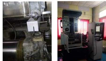
Fig 5 Wire Cut EDM Machine
