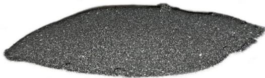
Fig 3 Silicon Carbide Powder
