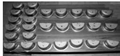
Fig.3 Cups sectioned at middle.
