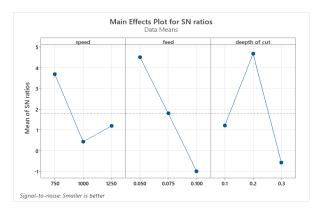
The response graphs given in elucidate the variation of surface roughness with the turning parameters. The ideal machining conditions are shown in these figures, along with the relative effects of the turning parameter on responses (the gradient of the line). The gradient of the line connecting the different
