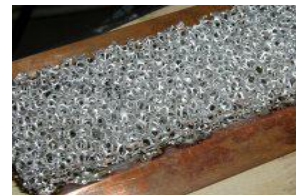
Fig 1. Open cell metal foam sample [5]
