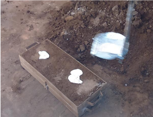
Fig. 3. Filling of molten Al in to the sand mould
