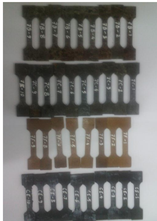
Fig. 5 JANNAF samples for Basalt, Carbon fiber, Fiber Glass and Carbon / Epoxy
