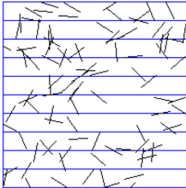
Figure 6. Buffon's Needle: after N tosses, the estimate for pi is (2N/X) , where X is the number of times the needle intersects a line (Harrison et al., 2010)
