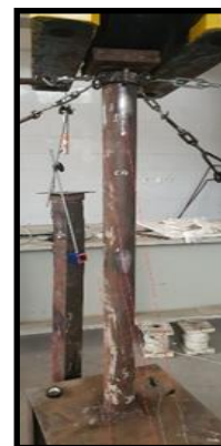
Figure (9) the locations of (LVDT)
