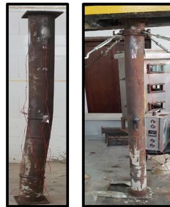
Figure (11) failure shape of (Cf)
