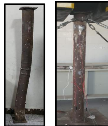
Figure (12) failure shape of (Cs)
