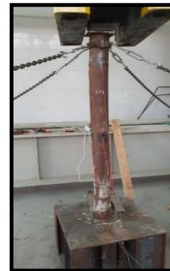
Figure (8) method of fixing cylinder column
