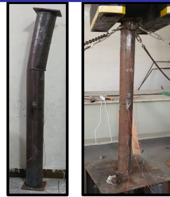
Figure (10) failure shape of (Ch)
