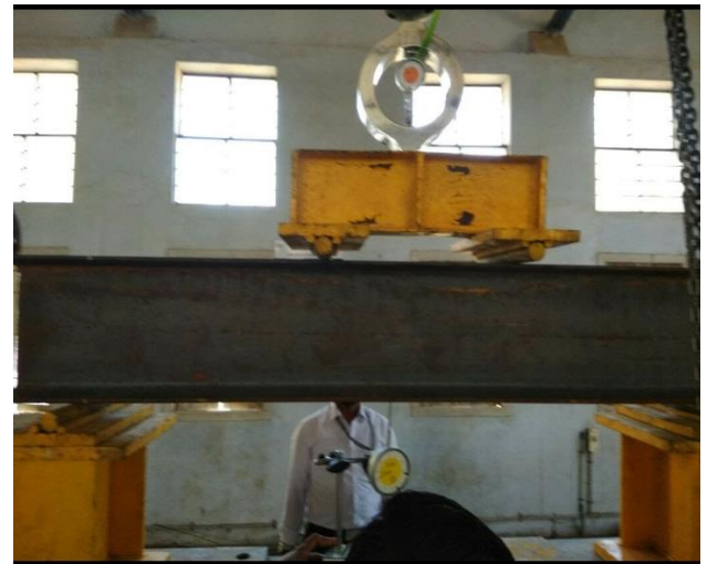
Fig.2: I-sectional beam loaded on the demec loading frame
