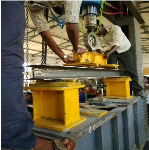
Fig.4: Double channelled section placed on demec loading frame
