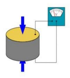
This gives piezoelectric sensors ruggedness, an extremely high natural frequency and an excellent linearity over a wide amplitude range.
