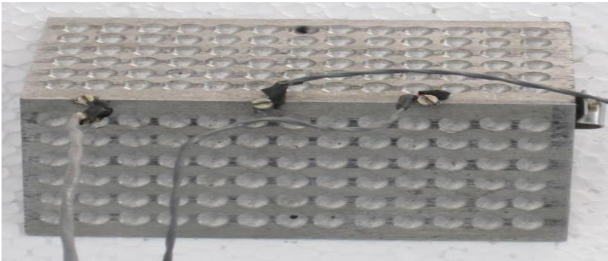
Fig3:- dimpled fin surface (triangular long fin bar)
