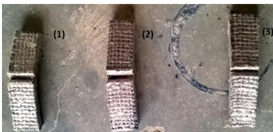
Fig 3: Impact test specimen after impact test
