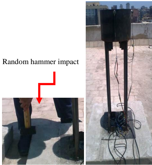
Figure 1. The mounted reference accelerometers, roving sensors and random hammer impact at the base
