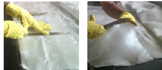
Fig:2 Cutting of fibers to the size 300 X 300 mm
