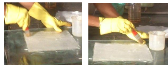
Fig: 3.layer by layer building of laminates
