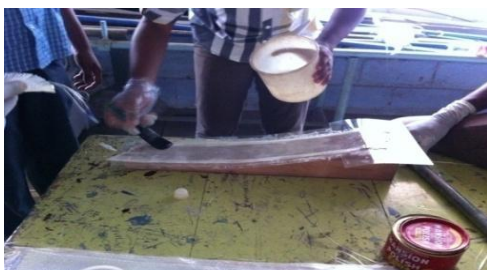
Fig.13 Epoxy/Hardener mixture applied over fiber sheet
