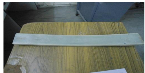
Fig.15 Prototype after trimming the sides
