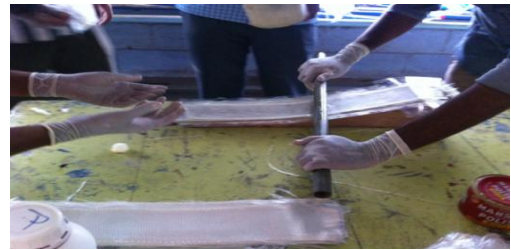
Fig.14 Squeezing out extra Epoxy (Compaction)
