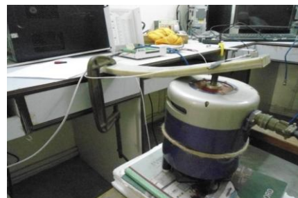
Fig.21 Forced Vibration Setup (Harmonic Exciter)
