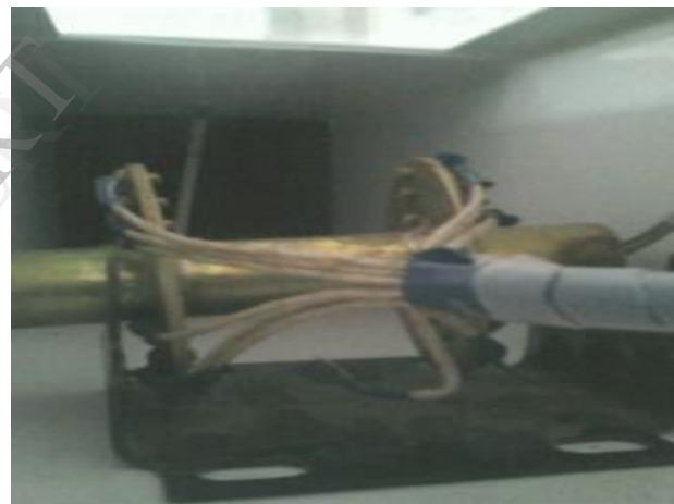
Figure 2: Elliptical fin set up with thermocouple locations
