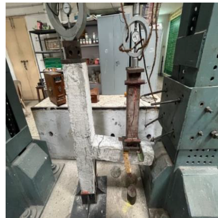
Fig. 8.1.2 Test Setup of Steel Fibre Beam and column joint
