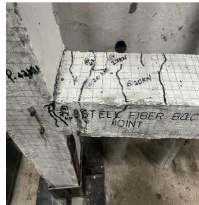
8.1.4 Test Setup of Steel Fibre B&C Joint
