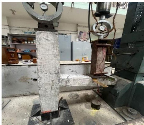
8.1.3 Test Setup of Conventional B&C joint
