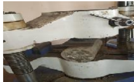
Fig 2. Cylinder Split tensile testing
