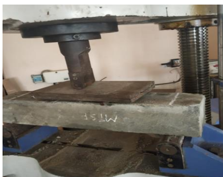
Fig 3 : Testing Modulus of rupture in prism
