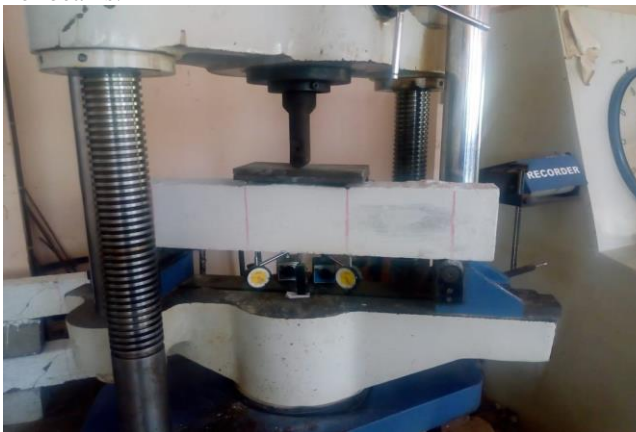
Fig 4: Testing RCC Beams
