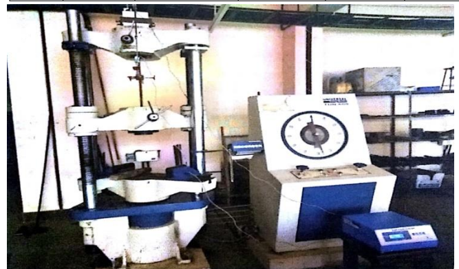
Fig 5: Pull out testing set up
