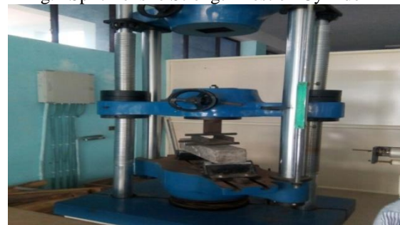
Fig.3 Specimen under Flexural Strength Test
