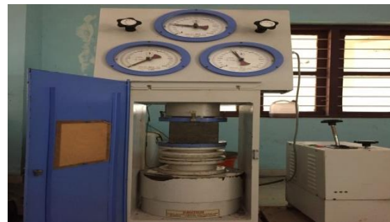
Fig.1 Compressive Strength Test on Cube
