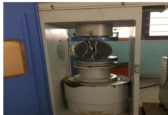
Fig.2 Split Tensile Strength Test on Cylinder
