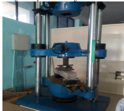
Fig.2 Flexural Strength Test on Beam
