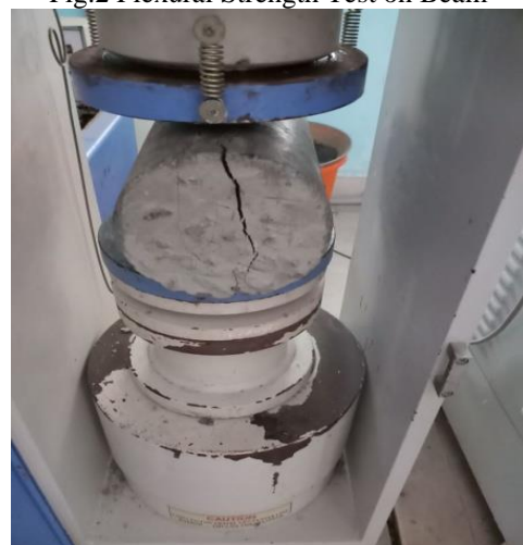
Fig.3 Split Tensile Strength Test on Cylinder
