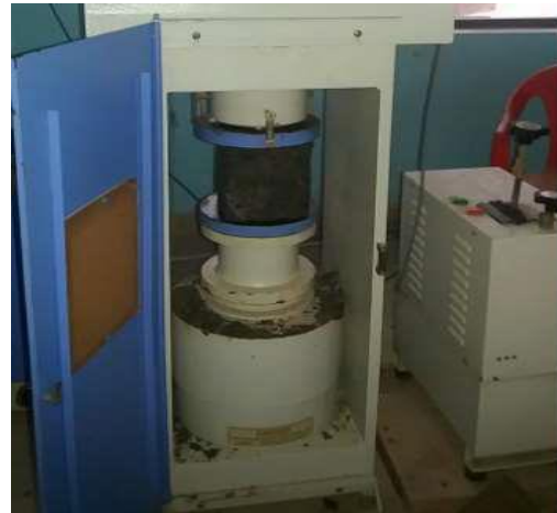
Fig.1 Compressive Strength Test on cube
