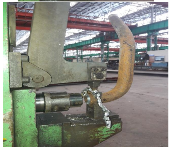
New Tool holder used for chamfering bend tubes with minimum arm length
