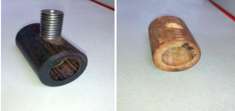
Fig 2: Main body made of rose wood and sapota wood respectively COLD TUBE:
