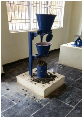
Fig.5 Compaction Factor Test
