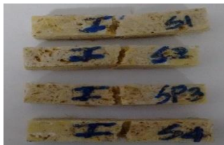
Fig 5.3 Impact load comparison of different composite Specimens
