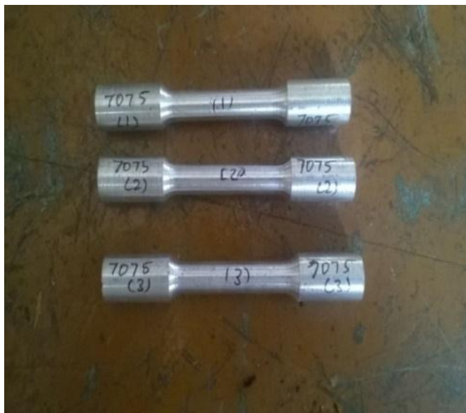
Fig.4. Specimens before tensile test
