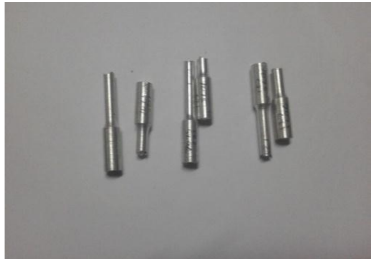
Fig.5. Specimens before tensile test
