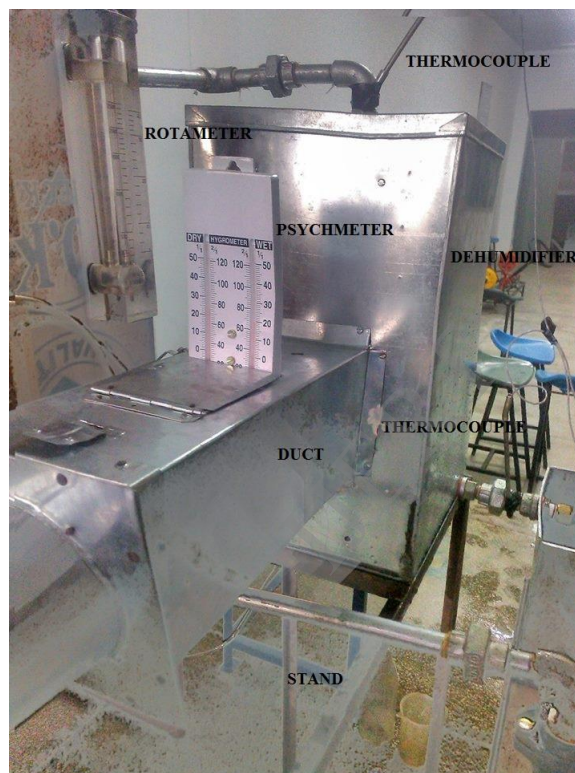
Figure 1. Experimental set up of cross flow dehumidifier.
