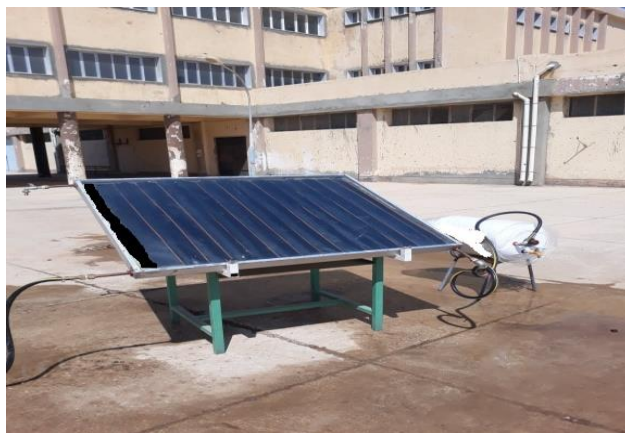
Figure (2) shown the first experiment of flow water inside the collector
