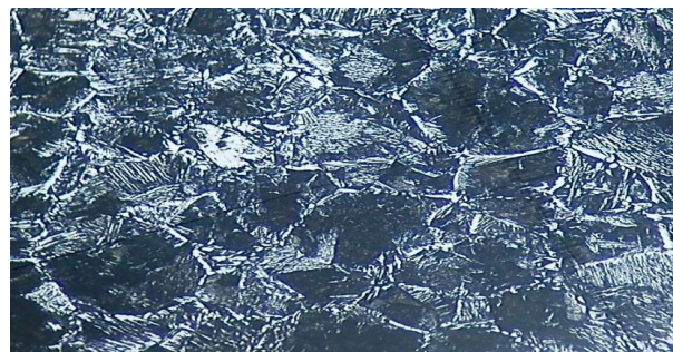
Fig 6 Heat Affected Zone at 100X
