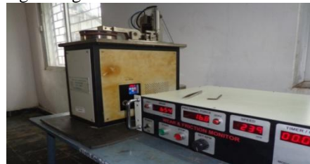
Fig 4 Wear test rig with data acquisition system
