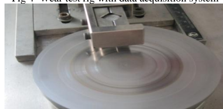
Fig 5: Wear test rig with specimen
