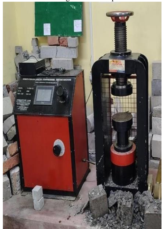
Fig. 4 Cube compressive strength test and compression testing machine setup
