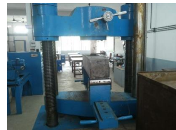
Fig 3: Flexural strength test on SFRC specimen
