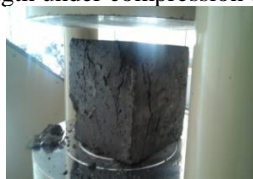
Fig 1: Compression test on SFRC specimen
