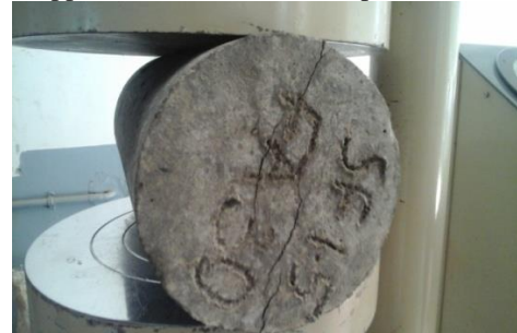
Fig 2: Split tensile strength test on SFRC specimen
