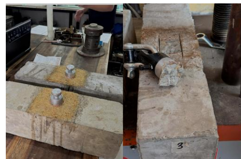
Fig. 13: Bond strength testing setup of coconut husk fiber-epoxy retrofitted beams using the ASTM D7522 pull-off method
