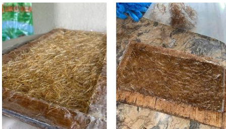
Fig. 11: Fabrication of alkali-treated coconut husk fiber-epoxy composite coupons for tensile testing according to ASTM D3039
