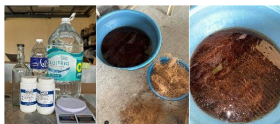
Fig. 3: Alkaline treatment of coconut husk fibers through immersion in 5% NaOH solution
