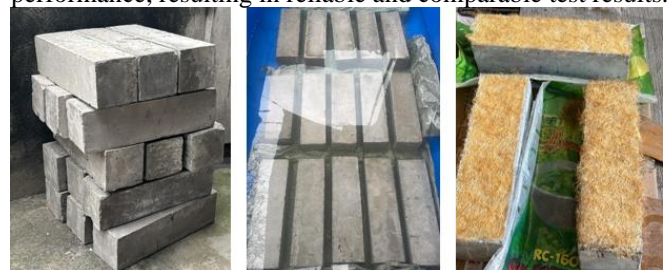
Fig. 10: Demolding, curing, and retrofitting of beam specimens with coconut husk fiber reinforcement prior to mechanical testing
