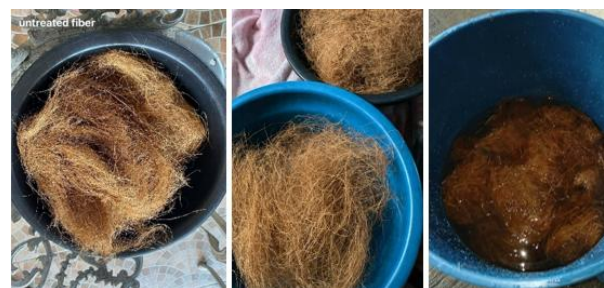
Fig. 2: Washing and Manual Cleaning of Raw Coconut Husk Fibers Prior to External Bonding Application
