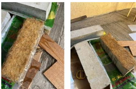
Fig. 5: Application of additional epoxy to fully coat the externally bonded coconut husk fibers
