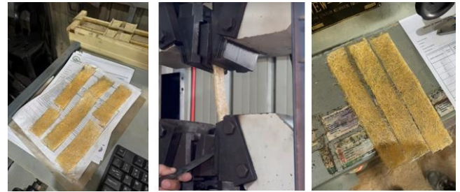
Fig. 12: Tensile testing setup of coconut husk fiber-epoxy composite specimens using a Universal Testing Machine
