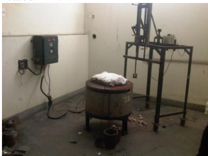
Fig 1. Furnace with stirring apparatus
