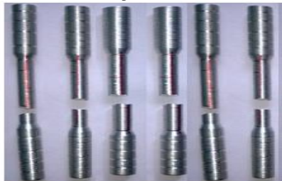
37mm Diameter Specimen after tensile test
