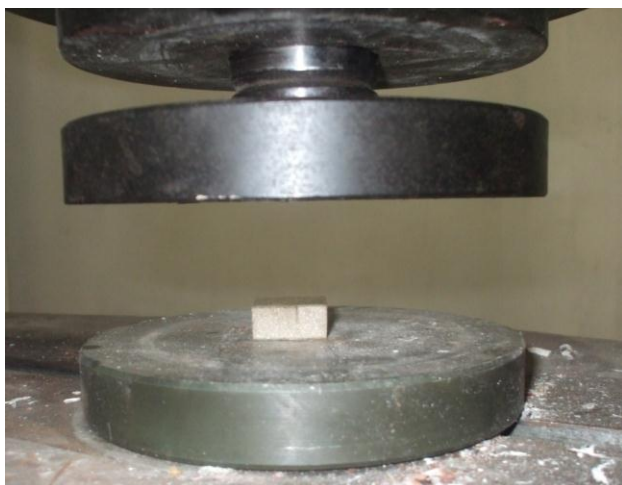
Figure 2: Flatwise compression test set up
